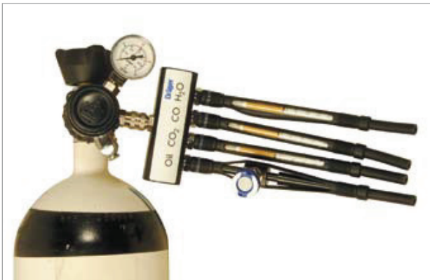
Measuring the air quality directly at the breathing air cylinder
