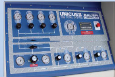
Hinged Cascade Fill Control Panel with Air Flow Schematic
